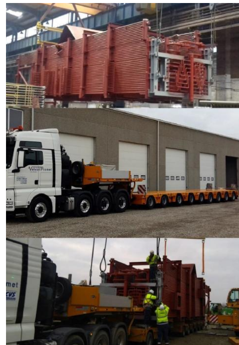
Fig. 1 Steam boiler module transport
