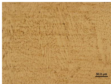
Fig. 10 Microstructure in the area of mixing the cladding metal Dievar and NiCu7
