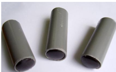
Fig. 2 Cartridges charged with non-detonating chemical mixture [2,6]
