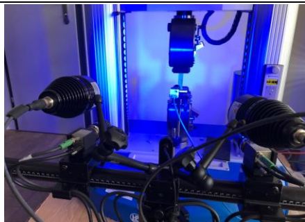
Fig. 1 Equipment during 2D and 3D DIC test.
