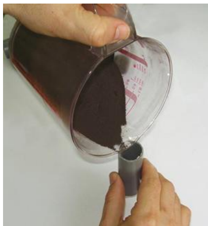
Fig. 1 Charging the cartridges with non-detonating chemical mixture [2,6]
