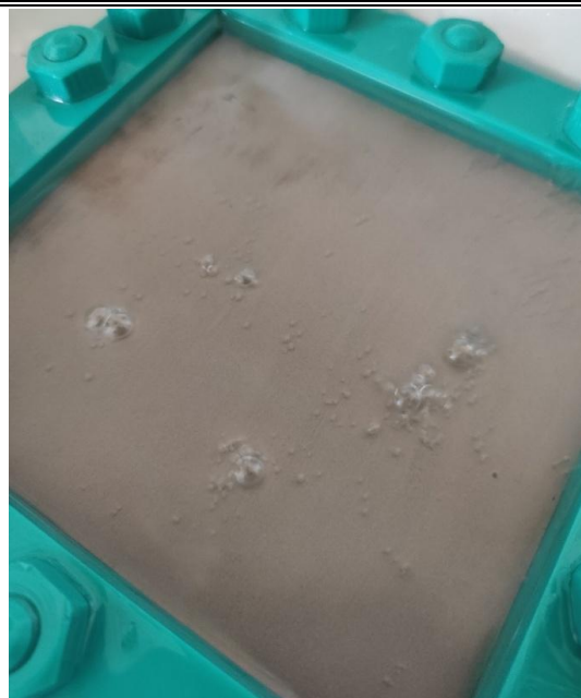
Fig.3 Determination of the maximum pore size by the bubble method.
