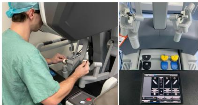
Fig. 1 The da Vinci Xi Model - Surgeon Console [1]
