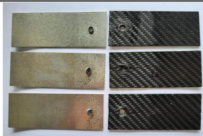
Fig. 13 Appearance of Al - PP CF substrates after load capacity test
