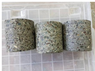
Photo 13 WS sample's general view after 5 cycles, zero mass lost
