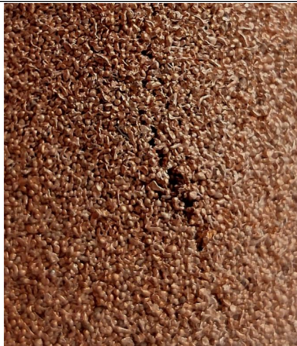
Fig. 4 Initial stage of crack formation on the outer surface of a curved sample.
