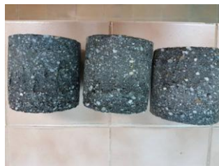
Photo 14 DS sample's general view after 5 cycles, mass lost
