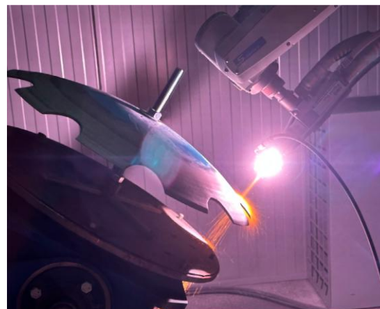
Figure 1. Atmospheric plasma jet thermal spraying coating process
