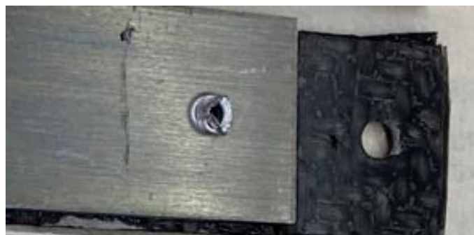
b) failure mode of AIOS-PA6GF joint
