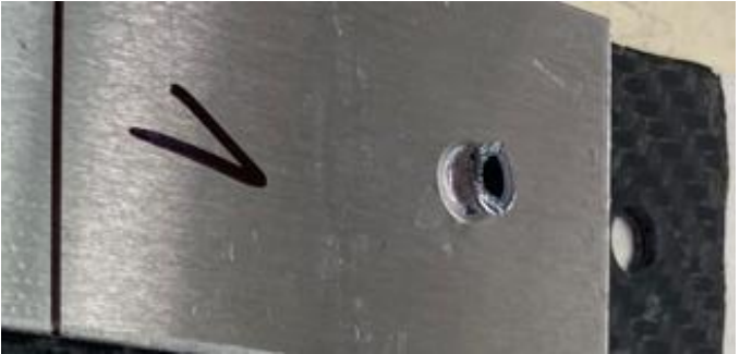
b) failure mode of Al-PA6CF joint
