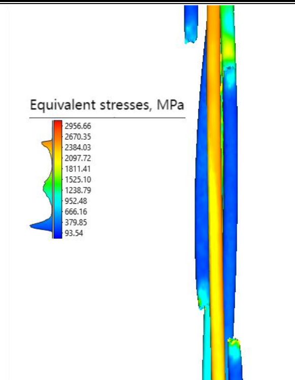
Fig. 2 Results of modeling of metal cord breakage
