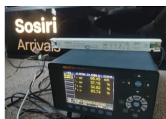
Fig. 2. Testing the panel power supply
