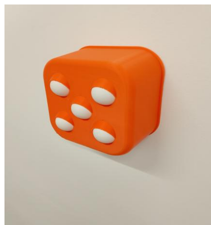
Fig. 4 A prototype of the developed innovative product with five valve bodies and spherical closing members with diameter of 40 millimeter.
