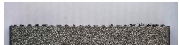
Fig. 4 Detailed view of burr formation at the groove edge
