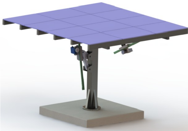
Fig. 3 3D CAD model of the single-pole dual-axis tracking system
